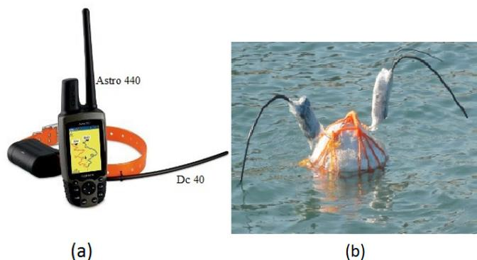
Figure 2. GPS receiver Garmin Astro 440 and a transmitter DC 40 (a) and a drifter buoy in water (b).
