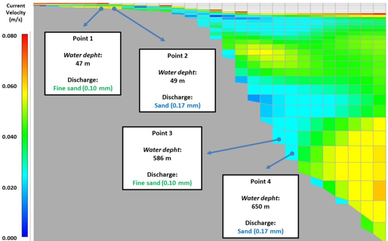
Figure 2. Representation of the vertical sections in the hydrodynamic model, with current velocities along the water column, and sediment discharge points.
