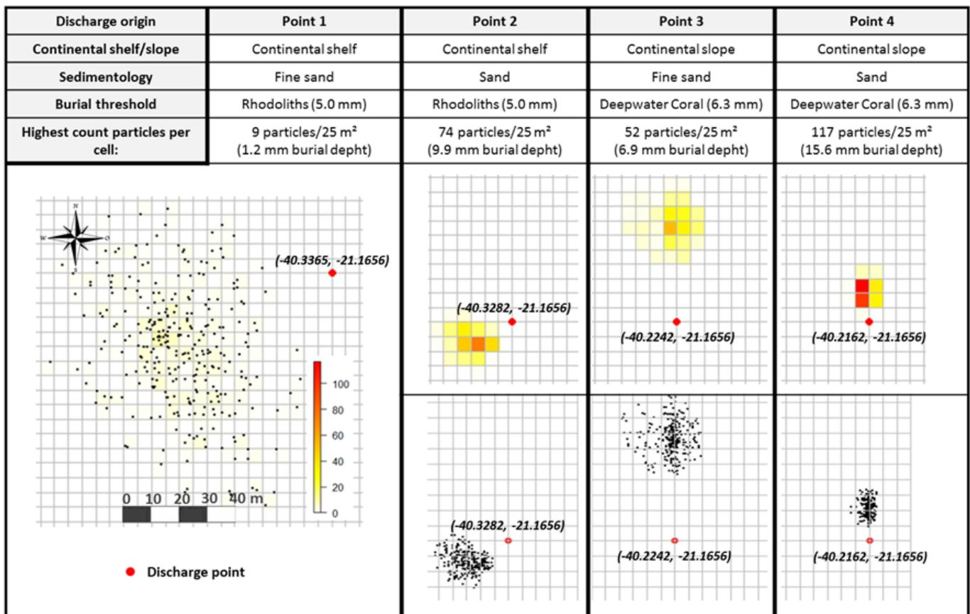
Figure 3. Particle dispersion and deposition results from the Lagrangian model. Discharges points with the respective geographical coordinates.
