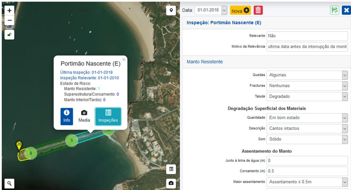
Figure 24. ANOSOM\_WEB interface used for populating the visual inspection database.
