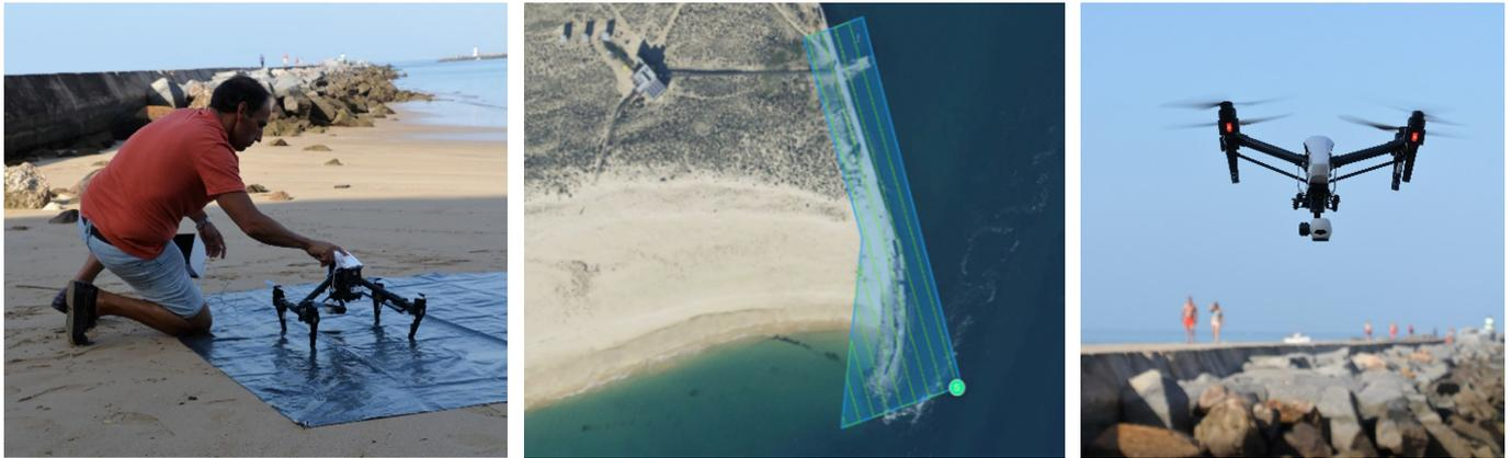
Figure 13. Preparing an UAV flight (left), with flight plan (middle), and beginning of the flight survey (right).
