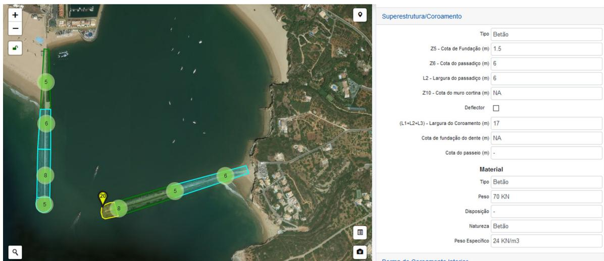
Figure 25. Searching in ANOSOM\_WEB interface for geometrical characteristics and materials.
