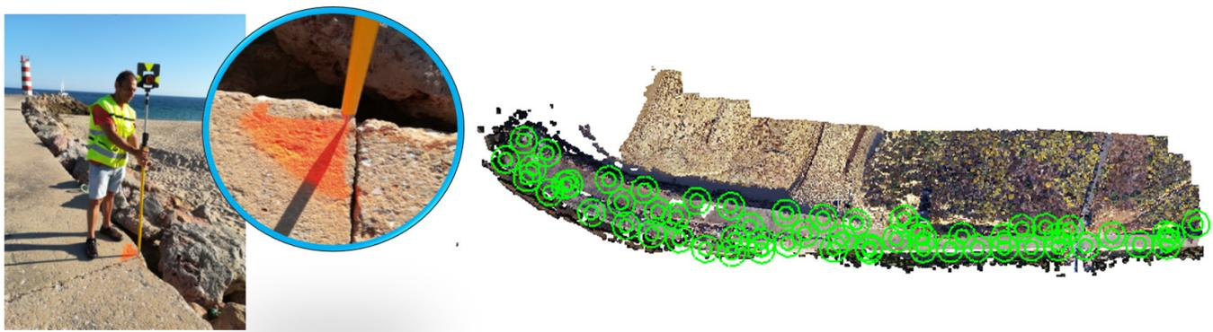
Figure 14. Survey of Ground Control Points on the superstructure and on one of the units of the armour layer.
