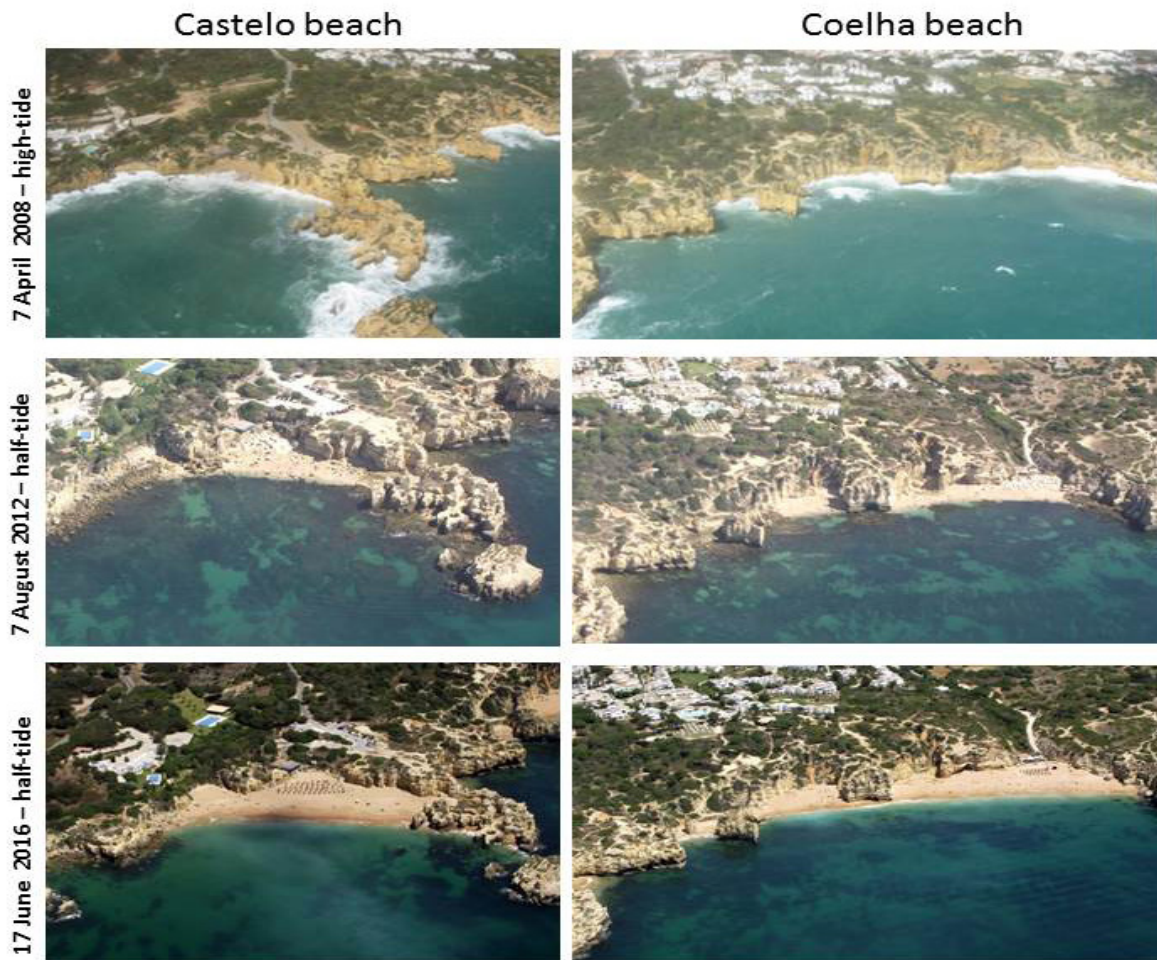
Figure 3. Castelo and Coelha beaches under storm conditions at high spring tide (7 Apr 2008, upper panel), under average summer wave conditions at half-tide before beach nourishment (7 Aug 2012, central panel) and under average summer wave conditions at half-tide after beach nourishment (17 Jun 2016, lower panel). Photos by the author.
