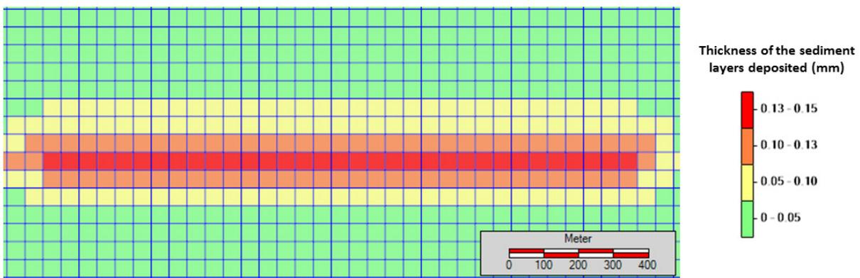
Figure 7. Seabed top view in the Case Study 2 transect region: simulated sediment layer deposited in the continental slope by the single-rig trawling operation in Campos Basin.
