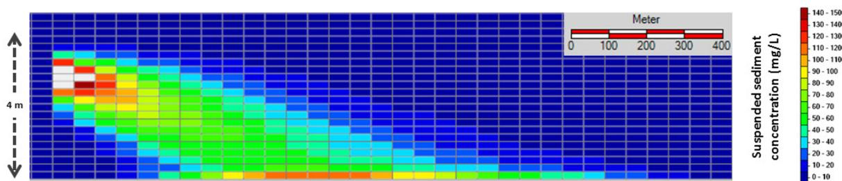
Figure 4. Vertical cut along Case Study 1 transect: simulated suspended sediment concentration from the double-rig trawling operation in the continental shelf of the Campos Basin.
