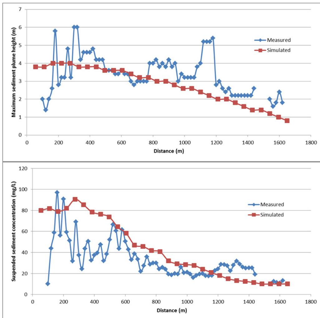
Figure 3. Measured and simulated longitudinal maximum sediment plume height (up) and suspended sediment concentrations in the water column (down) originated by the bottom trawling operation (Mengual *et al.*, 2016).
