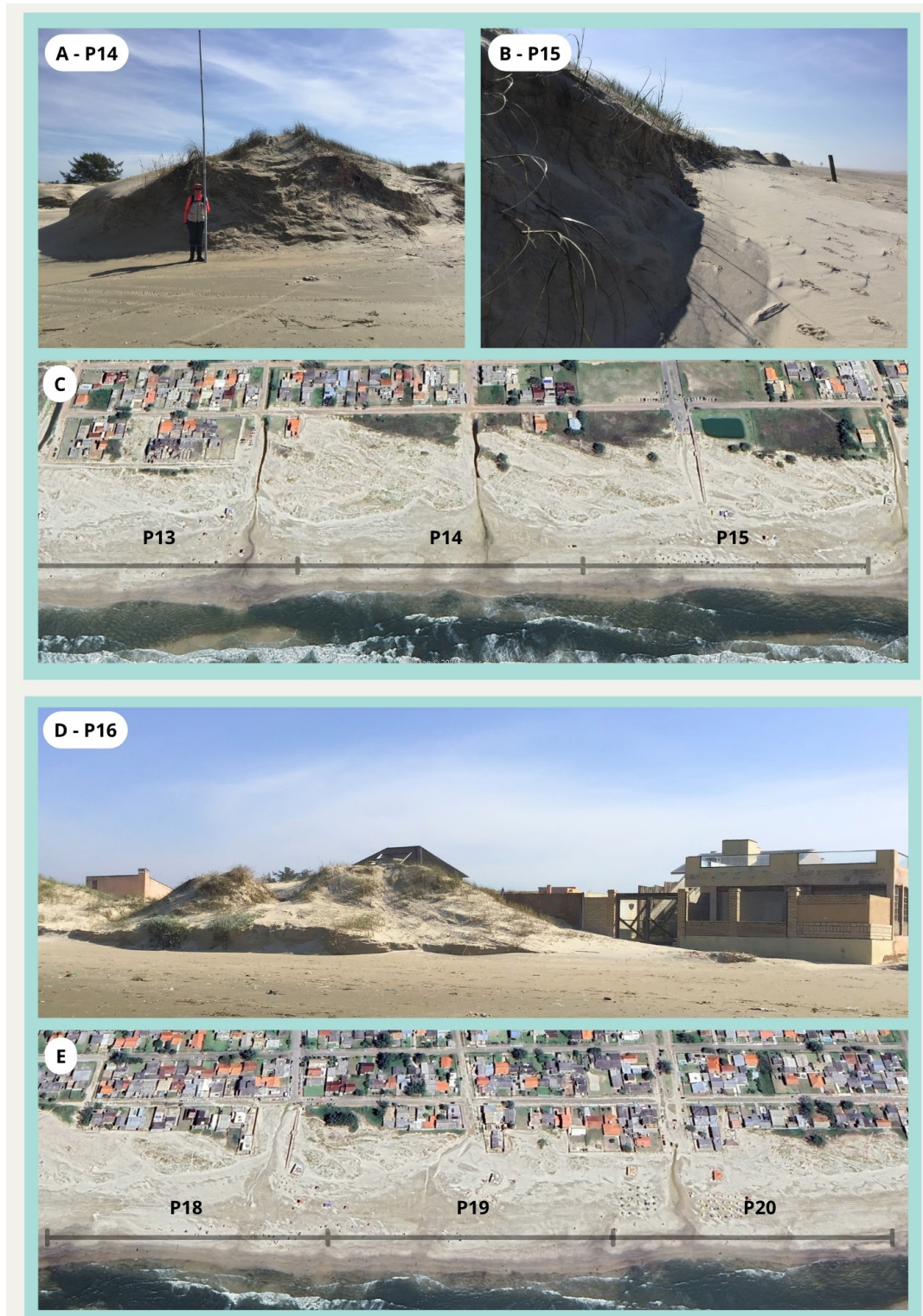
Figure 6: Records of sampling units with dunes characterized by steep slopes and erosional scarps. A-C: units from Cluster 2, highlighting the low percentage of impermeable surface within 200 meters inland from the shoreline. D-E: units from Cluster 3, characterized by a higher percentage of impermeable coverage in the same adjacent area. E - Google Earth Pro Satellite image (June 2023) of sampling unit P18-P20 from Cluster 3.
